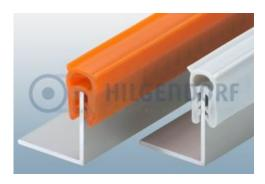
Edge protection profiles are used to protect against sharp-edged parts and are clamping automatically because of their geometry, so that no adhesives will be necessary. With the aid of additional embedded steel clamp strap or wire carrier a firm fit will be achieved. Edge protection profiles are manually mounted on the edge to be protected.
